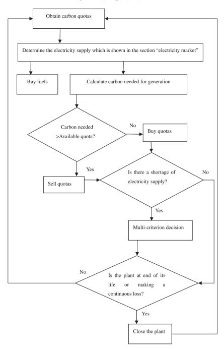
Fig. 2. Flow chart of power producers' actions.
